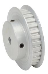
SureMotion timing pulley, aluminum, 1/5in XL pitch, 30 tooth, 1.91in pitch diameter, 1/4in bore, hub with flanges. For use with 1/4in wide belt.
