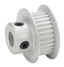
SureMotion timing pulley, aluminum, 0.08in MXL pitch, 30 tooth, 0.764in pitch diameter, 1/4in bore, hub with flanges. For use with 1/4in wide belt.
