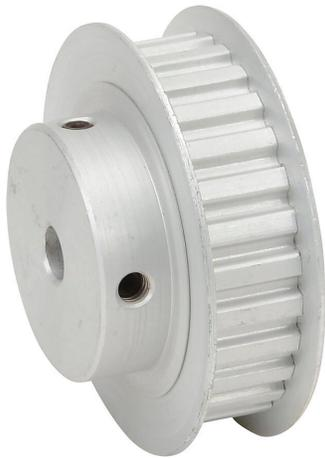
SureMotion timing pulley, aluminum, 1/5in XL pitch, 28 tooth, 1.783in pitch diameter, 1/4in bore, hub with flanges. For use with 3/8in wide belt.
