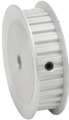
SureMotion timing pulley, aluminum, 1/5in XL pitch, 28 tooth, 1.783in pitch diameter, 1/4in bore, no hub with flanges. For use with 3/8in wide belt.
