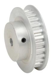
SureMotion timing pulley, aluminum, 1/5in XL pitch, 28 tooth, 1.783in pitch diameter, 1/4in bore, hub with flanges. For use with 1/4in wide belt.
