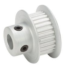
SureMotion timing pulley, aluminum, 0.08in MXL pitch, 28 tooth, 0.713in pitch diameter, 1/4in bore, hub with flanges. For use with 1/4in wide belt.
