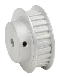
SureMotion timing pulley, aluminum, 1/5in XL pitch, 26 tooth, 1.655in pitch diameter, 1/4in bore, hub with flanges. For use with 3/8in wide belt.
