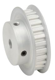
SureMotion timing pulley, aluminum, 1/5in XL pitch, 26 tooth, 1.655in pitch diameter, 1/4in bore, hub with flanges. For use with 1/4in wide belt.
