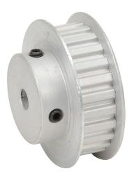
SureMotion timing pulley, aluminum, 1/5in XL pitch, 25 tooth, 1.592in pitch diameter, 1/4in bore, hub with flanges. For use with 3/8in wide belt.
