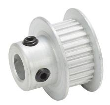
SureMotion timing pulley, aluminum, 0.08in MXL pitch, 25 tooth, 0.637in pitch diameter, 1/4in bore, hub with flanges. For use with 1/4in wide belt.
