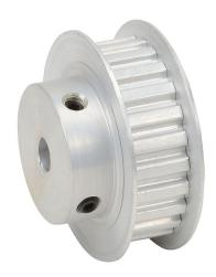
SureMotion timing pulley, aluminum, 1/5in XL pitch, 24 tooth, 1.528in pitch diameter, 1/4in bore, hub with flanges. For use with 3/8in wide belt.
