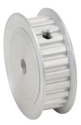
SureMotion timing pulley, aluminum, 1/5in XL pitch, 24 tooth, 1.528in pitch diameter, 1/4in bore, no hub with flanges. For use with 3/8in wide belt.
