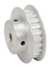
SureMotion timing pulley, aluminum, 1/5in XL pitch, 24 tooth, 1.528in pitch diameter, 1/4in bore, hub with flanges. For use with 1/4in wide belt.
