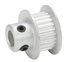
SureMotion timing pulley, aluminum, 0.08in MXL pitch, 24 tooth, 0.611in pitch diameter, 1/4in bore, hub with flanges. For use with 1/4in wide belt.
