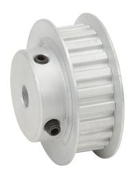
SureMotion timing pulley, aluminum, 1/5in XL pitch, 23 tooth, 1.464in pitch diameter, 1/4in bore, hub with flanges. For use with 3/8in wide belt.
