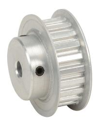
SureMotion timing pulley, aluminum, 1/5in XL pitch, 22 tooth, 1.401in pitch diameter, 1/4in bore, hub with flanges. For use with 3/8in wide belt.
