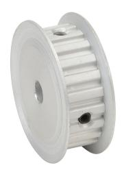
SureMotion timing pulley, aluminum, 1/5in XL pitch, 22 tooth, 1.401in pitch diameter, 1/4in bore, no hub with flanges. For use with 3/8in wide belt.
