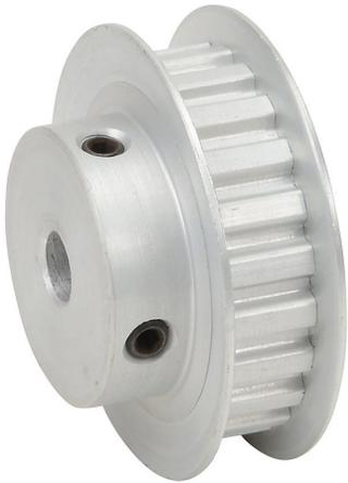
SureMotion timing pulley, aluminum, 1/5in XL pitch, 22 tooth, 1.401in pitch diameter, 1/4in bore, hub with flanges. For use with 1/4in wide belt.
