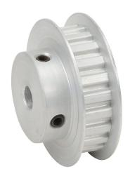
SureMotion timing pulley, aluminum, 1/5in XL pitch, 22 tooth, 1.401in pitch diameter, 1/4in bore, hub with flanges. For use with 1/4in wide belt.
