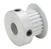
SureMotion timing pulley, aluminum, 0.08in MXL pitch, 22 tooth, 0.56in pitch diameter, 1/4in bore, oversize hub with flange. For use with 1/4in wide belt.
