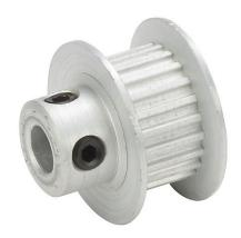
SureMotion timing pulley, aluminum, 0.08in MXL pitch, 22 tooth, 0.56in pitch diameter, 3/16in bore, hub with flanges. For use with 1/4in wide belt.
