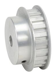
SureMotion timing pulley, aluminum, 3/8in L pitch, 22 tooth, 2.626in pitch diameter, 1/2in bore, hub with flanges. For use with 1/2in wide belt.
