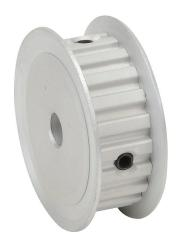
SureMotion timing pulley, aluminum, 1/5in XL pitch, 21 tooth, 1.337in pitch diameter, 1/4in bore, no hub with flanges. For use with 3/8in wide belt.
