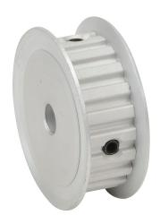
SureMotion timing pulley, aluminum, 1/5in XL pitch, 21 tooth, 1.337in pitch diameter, 1/4in bore, no hub with flanges. For use with 3/8in wide belt.
