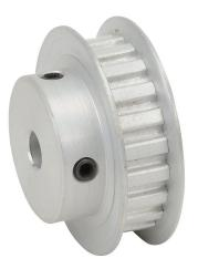
SureMotion timing pulley, aluminum, 1/5in XL pitch, 21 tooth, 1.337in pitch diameter, 1/4in bore, hub with flanges. For use with 1/4in wide belt.
