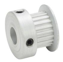
SureMotion timing pulley, aluminum, 0.08in MXL pitch, 21 tooth, 0.535in pitch diameter, 1/4in bore, oversize hub with flange. For use with 1/4in wide belt.
