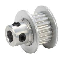
SureMotion timing pulley, aluminum, 0.08in MXL pitch, 21 tooth, 0.535in pitch diameter, 3/16in bore, hub with flanges. For use with 1/4in wide belt.
