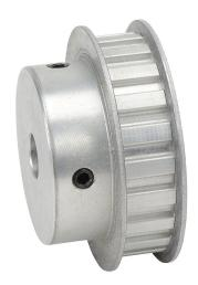
SureMotion timing pulley, aluminum, 3/8in L pitch, 21 tooth, 2.507in pitch diameter, 1/2in bore, hub with flanges. For use with 1/2in wide belt.
