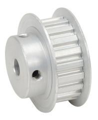
SureMotion timing pulley, aluminum, 1/5in XL pitch, 20 tooth, 1.273in pitch diameter, 1/4in bore, hub with flanges. For use with 3/8in wide belt.
