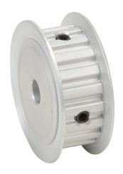
SureMotion timing pulley, aluminum, 1/5in XL pitch, 20 tooth, 1.273in pitch diameter, 1/4in bore, no hub with flanges. For use with 3/8in wide belt.
