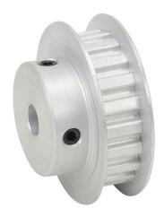
SureMotion timing pulley, aluminum, 1/5in XL pitch, 20 tooth, 1.273in pitch diameter, 1/4in bore, hub with flanges. For use with 1/4in wide belt.
