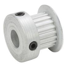
SureMotion timing pulley, aluminum, 0.08in MXL pitch, 20 tooth, 0.509in pitch diameter, 1/4in bore, oversize hub with flange. For use with 1/4in wide belt.
