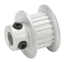
SureMotion timing pulley, aluminum, 0.08in MXL pitch, 20 tooth, 0.509in pitch diameter, 3/16in bore, hub with flanges. For use with 1/4in wide belt.
