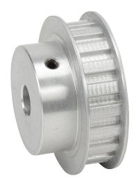
SureMotion timing pulley, aluminum, 3/8in L pitch, 20 tooth, 2.387in pitch diameter, 1/2in bore, hub with flanges. For use with 1/2in wide belt.
