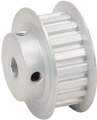
SureMotion timing pulley, aluminum, 1/5in XL pitch, 19 tooth, 1.21in pitch diameter, 1/4in bore, hub with flanges. For use with 3/8in wide belt.
