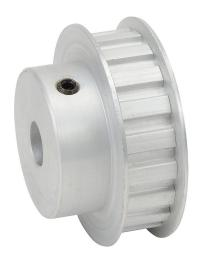
SureMotion timing pulley, aluminum, 3/8in L pitch, 19 tooth, 2.268in pitch diameter, 1/2in bore, hub with flanges. For use with 1/2in wide belt.
