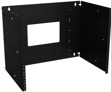
Hammond hinged wall-mount rack, 8U, 19in rack width, 12 to 18in depth, 100lb capacity, carbon steel, black, powder coat finish.
