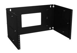
Hammond hinged wall-mount rack, 6U, 19in rack width, 12 to 18in depth, 100lb capacity, carbon steel, black, powder coat finish.
