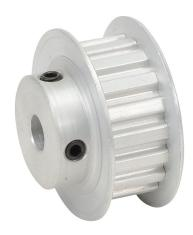
SureMotion timing pulley, aluminum, 1/5in XL pitch, 18 tooth, 1.146in pitch diameter, 1/4in bore, hub with flanges. For use with 3/8in wide belt.
