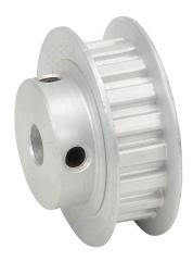
SureMotion timing pulley, aluminum, 1/5in XL pitch, 18 tooth, 1.146in pitch diameter, 1/4in bore, hub with flanges. For use with 1/4in wide belt.
