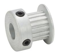
SureMotion timing pulley, aluminum, 0.08in MXL pitch, 18 tooth, 0.458in pitch diameter, 1/4in bore, oversize hub with flange. For use with 1/4in wide belt.
