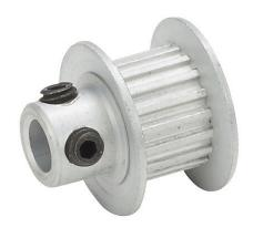
SureMotion timing pulley, aluminum, 0.08in MXL pitch, 18 tooth, 0.458in pitch diameter, 3/16in bore, hub with flanges. For use with 1/4in wide belt.
