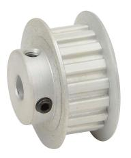
SureMotion timing pulley, aluminum, 1/5in XL pitch, 17 tooth, 1.082in pitch diameter, 1/4in bore, hub with flanges. For use with 3/8in wide belt.
