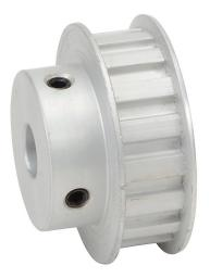
SureMotion timing pulley, aluminum, 3/8in L pitch, 17 tooth, 2.029in pitch diameter, 1/2in bore, hub with flanges. For use with 1/2in wide belt.
