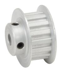
SureMotion timing pulley, aluminum, 1/5in XL pitch, 16 tooth, 1.019in pitch diameter, 1/4in bore, hub with flanges. For use with 3/8in wide belt.
