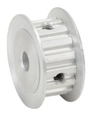
SureMotion timing pulley, aluminum, 1/5in XL pitch, 16 tooth, 1.019in pitch diameter, 1/4in bore, no hub with flanges. For use with 3/8in wide belt.
