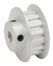
SureMotion timing pulley, aluminum, 1/5in XL pitch, 16 tooth, 1.019in pitch diameter, 1/4in bore, hub with flanges. For use with 1/4in wide belt.
