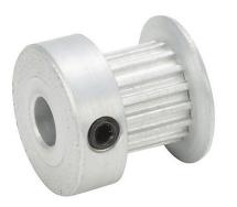
SureMotion timing pulley, aluminum, 0.08in MXL pitch, 16 tooth, 0.407in pitch diameter, 3/16in bore, oversize hub with flange. For use with 1/4in wide belt.
