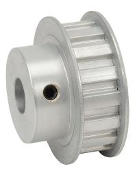
SureMotion timing pulley, aluminum, 3/8in L pitch, 16 tooth, 1.91in pitch diameter, 1/2in bore, hub with flanges. For use with 1/2in wide belt.
