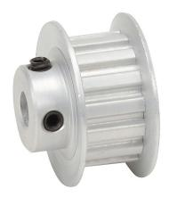
SureMotion timing pulley, aluminum, 1/5in XL pitch, 15 tooth, 0.955in pitch diameter, 1/4in bore, hub with flanges. For use with 3/8in wide belt.
