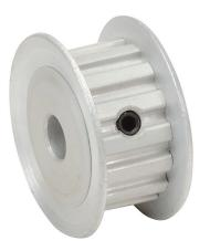
SureMotion timing pulley, aluminum, 1/5in XL pitch, 15 tooth, 0.955in pitch diameter, 1/4in bore, no hub with flanges. For use with 3/8in wide belt.
