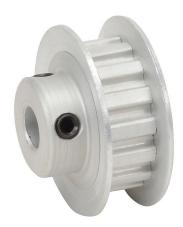
SureMotion timing pulley, aluminum, 1/5in XL pitch, 15 tooth, 0.955in pitch diameter, 1/4in bore, hub with flanges. For use with 1/4in wide belt.
